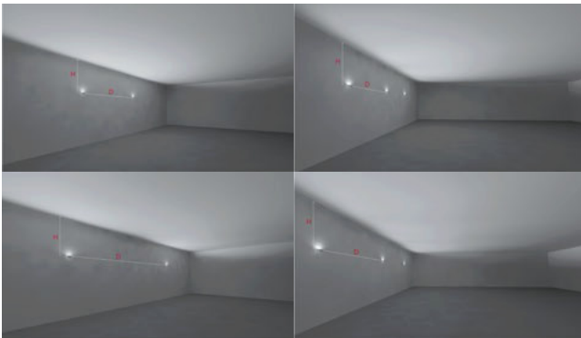
On the left is a comparison of the effects of horizontal wall washing H: D=1:2.5&1:4.5; Vertical wall washing on the right H: D=1:2&1:3 effect comparison
